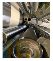
Coating of the paper with recyclable and compostable dispersion coating layer
