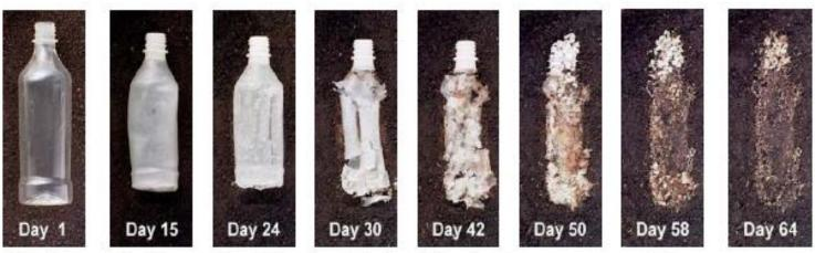
Biodegradation of a Bioplastic bottle during composting
