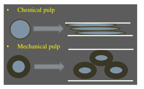
Chemical Pulp fibres are flexible and strong Mechanical Pulp fibres are rigid and bulky
